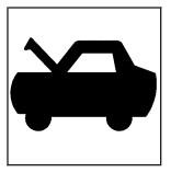
1. Pull the hood release lever with this symbol on it. It is located inside the vehicle on the lower left side of the instrument panel.
